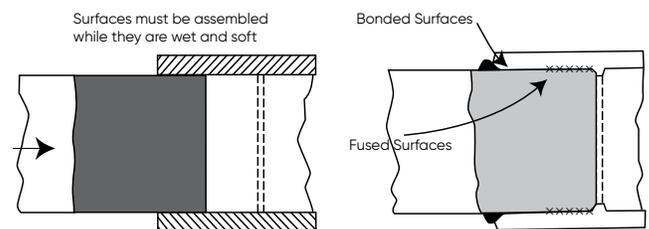
As the solvent dissipates, the solvent cement layer and the dissolved surfaces will dry and harden with a corresponding increase in joint strength. Completed joints must not be disturbed until they have properly set. See the Joint Set Schedule table for details.
