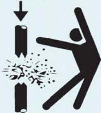
**NEVER** use this product or other rigid PVC/CPVC piping products for the transportation or storage of compressed air or gases, nor the testing of these systems using compressed air or gases.
