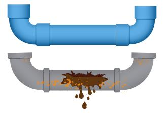
PVC does not corrode; most breaks are caused by corrosion
