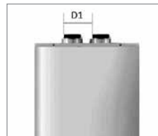
Figure 7: Vent Collar Spacing
