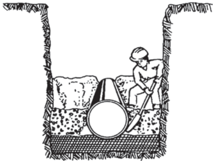
Get rid of voids under the pipe.
