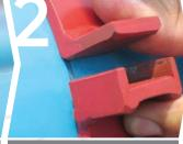
Position the Pipe Stop so that it just covers the insertion line.
