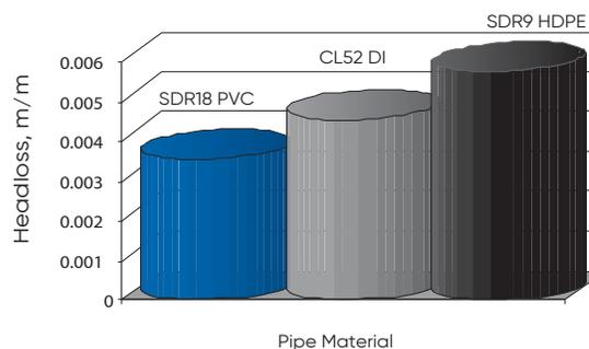
The 'C' factors obviously have a significant effect on flow rates. Comparing various materials it can be seen that PVC pipe has a much lower headloss at any given flow than other common piping materials.
